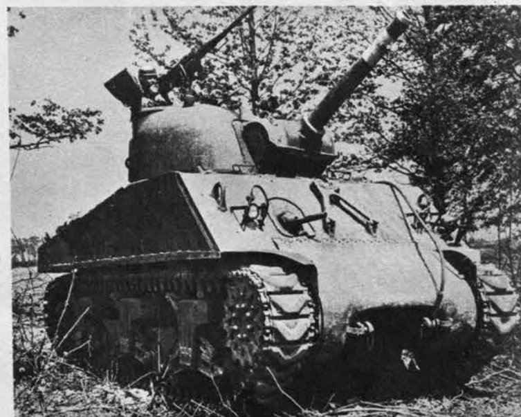
Heavy 105-mm. howitzer is one variation in M-4 armament. It requires a heavier gun mantlet than the standard 75 (above). The U. S. Third Army's Shermans used this howitzer in drive across France.
